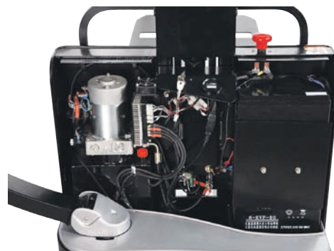
Built in charger and maintance free batteries
